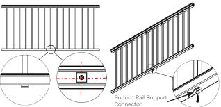
Note: For shorter sections, Remove an additional 8mm on both ends (16mm overall) for the bracket to fit between the rail and post. Trim the top and bottom rails to length.
