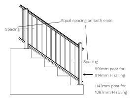
Note: During installation, please don't tilt the railing to the maximum angle repeatedly as this will scratch the powder coating on the pickets.
