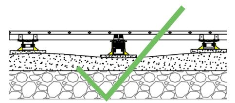
NewTechWood products shown above can be on pedestals or jacks if the surface is uneven. Consult with the pedestal or jack manufacturer before using the product to ensure its compatibility with NewTechWood's products.
