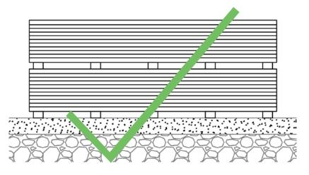
NewTechWood products shown above put on a flat surface on joists, this is the correct way for storage.
