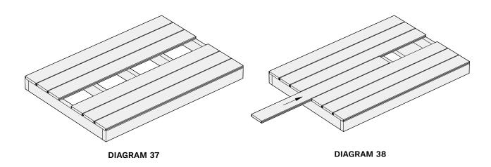
5 After the new board is in position insert the clips through the groove and into the correct position as shown in Diagram 39.
