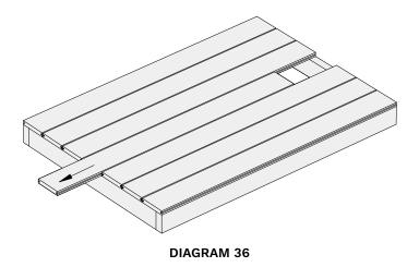
After the board is removed the new board can be inserted as shown below in Diagram 37 and 38.
