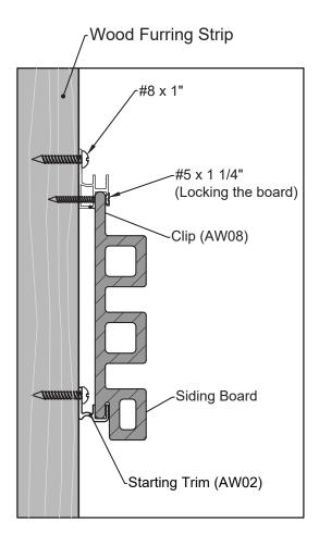
When installing horizontally, it is required to lock the Clip (AW08) at the middle of the board, as shown in **Diagram A1**.
