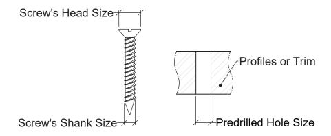
The predrilled hole size should be larger than the screw thread size, from 1/16" (1.5 mm) to 5 /64" (2 mm). Moreover, the predrilled hole size should also be smaller than the screw head size, at least 5/64" (2 mm). A washer can be applied if the predrilled hole size is smaller than the screw head size below 5/64" (2 mm).
